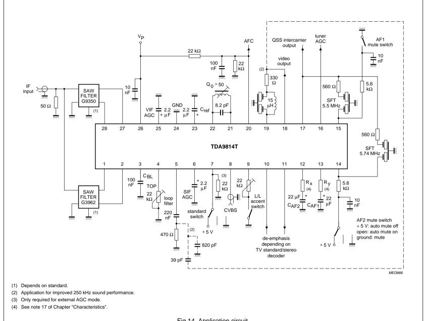
Fig.14 Application circuit.
