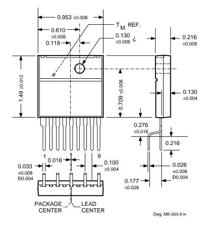
NOTE: Exact body and lead configuration at vendorÕs option within limits shown.
