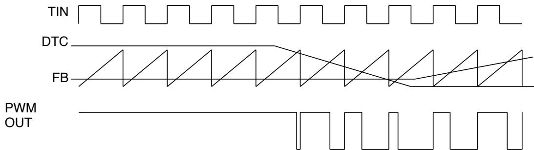
• PWM OUT ON Duty is fixed in the voltage of higher one between DTC terminal and FB terminal voltage.
