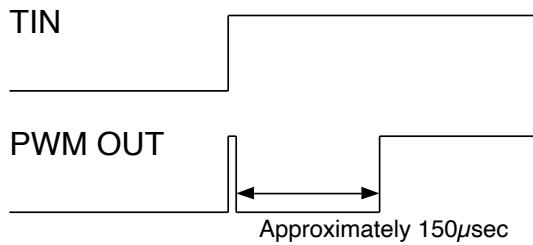
• Waveform at "L" was taken from "H", and having put TIN up (PWM output is fixed in "L", too when fix TIN terminal in "L".)
