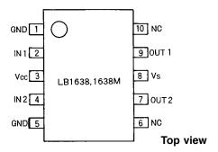
Note: both ground pins must be grounded.
