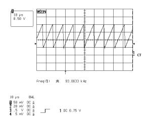
**Burst oscillator & burst dimming** :Timing capacitor BCT are charged by the reference current source, formed by the timing resistor Rt whose voltage is regulated at 1.25V. The sawtooth waveform charges up to 2V. Once reached, capacitors begin discharging down to 0.5V. Next timing capacitors start charging again and a new switching cycle begins. The burst dimming frequency can be programmed with adjusting the values of Rt and BCT. The burst dimming frequency can be calculated as below.
