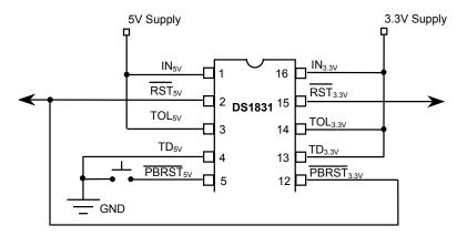
NOTE: The  $\overline{\text{RST}}_{5V}$  output is connected to the  $IN_{3.3V}$  via a 100 k $\Omega$  resistor in the push-button input and therefore does not require a pull-up resistor (an addition pull up can be used to accelerate responses). If an external pull up is used in this example it must be connected to the 3.3V power supply.
