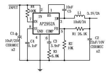
Figure 1. Typical Application Circuit
