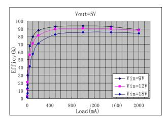
Figure 2. Typical Efficiency Curve
