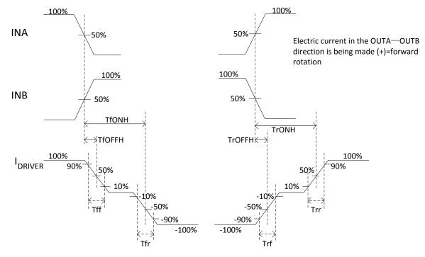
Fig.1 switching characteristics waveform
