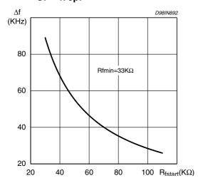
Figure 8. Typ. (fstart-fmin) vs. Rfstar @ Cf = 470pF
