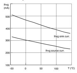
Figure 20. LVG Source and Sink Current vs. Temperature
