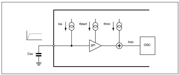
During the soft start time the current I<sub>SS</sub> charges the capacitor C<sub>SS</sub>, generating a voltage ramp which is delivered to a transconductance amplifier, as shown in fig. 4. Thus this voltage signal is converted in a growing current which is subtracted to I<sub>fstart</sub>. Therefore the current which drives the oscillator to set the frequency during the soft start is equal to:
