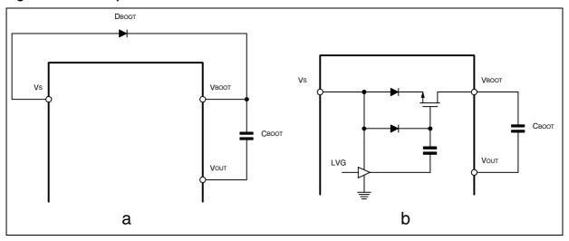
To drive the synchronised DMOS it is necessary a voltage higher than the supply voltage Vs. This voltage is obtained by means of an internal charge pump (fig. 11b).
