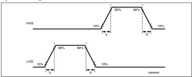
Figure 13. Dead Time and Duty Cycle Waveform Definition
