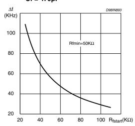
Figure 9. Typ. (fstart-fmin) vs. Rfstar @ Cf = 470pF
