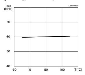
Figure 15. Typ. fstart vs. Temperature
