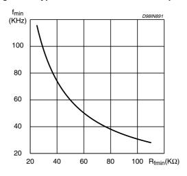
Figure 7. Typ. (fstart-fmin) vs. Rfstar @ Cf = 470pF
