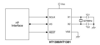
\*Note: The value of the capacity depends on how accurate the crystal is.
