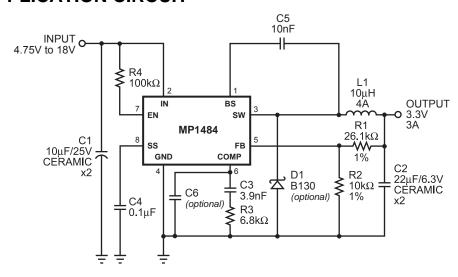
Figure 3—MP1484 with 3.3V Output, 22uF/6.3V Ceramic Output Capacitor
