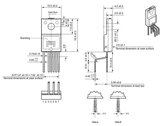
Gate burr: 0.3 mm (max.) Terminal core material: Cu
