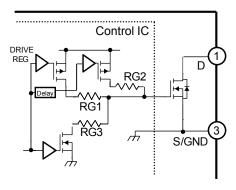
Figure 20. Step drive circuit
