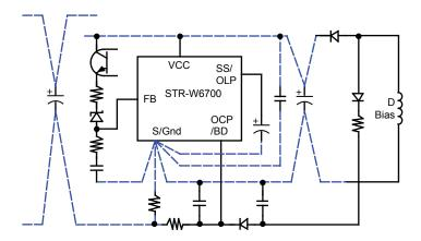
Figure 26. High frequency, high current loops
