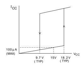
Figure 3. VCC pin current versus voltage
