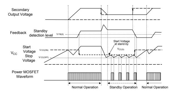
Figure 19. Quasi-resonant to bottom-skip operation timing
