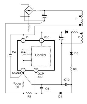
Figure 16. Quasi-resonant and delay circuit
