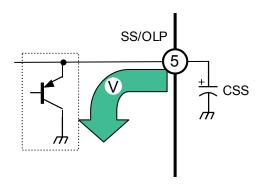
Figure 11. Reset circuit at power turn off
