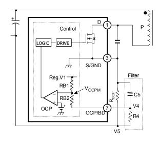
Figure 15. OCP functional block diagram
