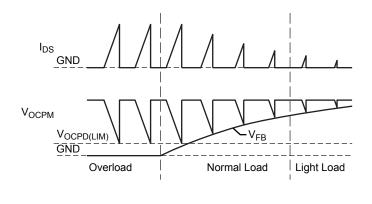
Figure 13. Constant-voltage control at fixed oscillation frequency (quasiresonant signal not available)
