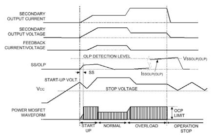
Figure 10. Timing at overload
