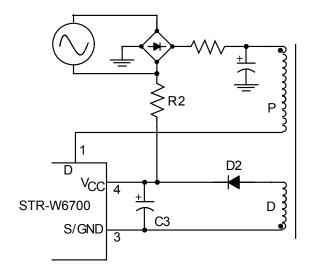
Figure 2. External start-up circuit.
