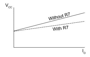
Figure 5. V<sub>CC</sub> versus I<sub>O</sub> (secondary load)
