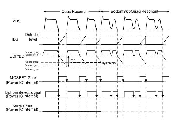
Figure 17. Quasi-resonant to bottom-skip operation timing
