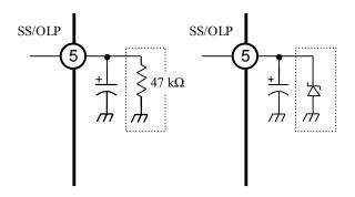
Figure 12. OLP deactivation circuit alternative configurations
