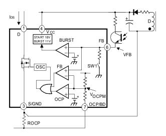
Figure 14. REG circuit functional block diagram
