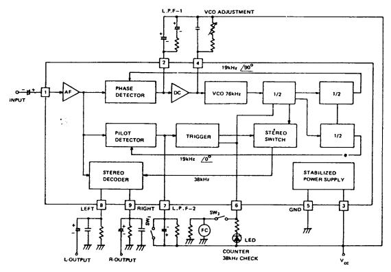
SW<sub>1</sub>: VCO STOP SWITCH SW<sub>2</sub>: J8kHz MONITOR SWITCH
