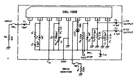
\* Each C<sub>6</sub> and C<sub>7</sub> is  $0.015\mu F$  for Demphasis (50  $\mu sec$ ) but  $0.022\mu F$  for (75 $\mu sec$ )
